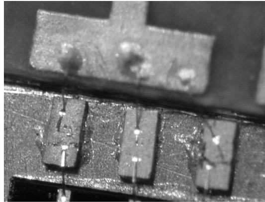
Figure 7: Epoxy on bonding deposition.
