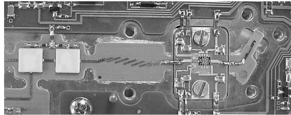
Figure 11: 25.7 GHz transmitter full production module.
