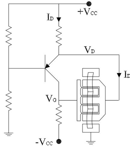
Figure 6: Active biasing network for PAE improvement and avoiding adjustments.
