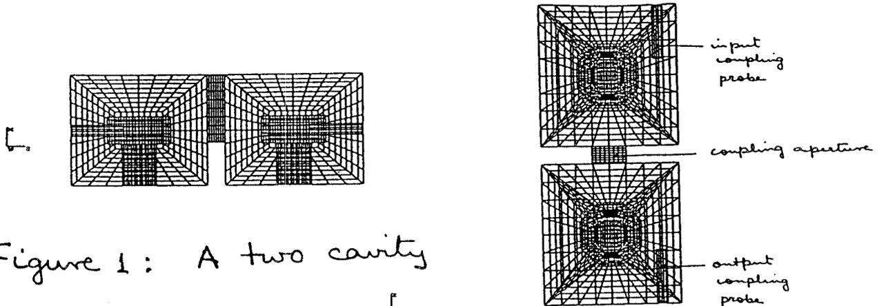
Figure 1: A two cavity coupled dielectric resonator
