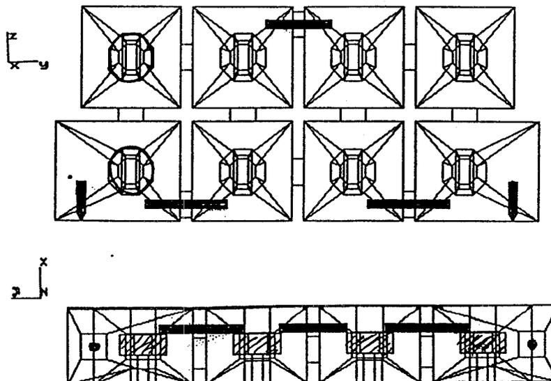
Figure 2: An eight cavity coupled dielectric resonator
